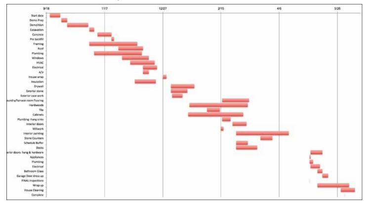
onstruction planning can help minimize costs by optimizing resource and equipment utilization. Even for small residential projects, you may have to lease the necessary equipment. On large commercial projects, leasing or buying specialized equipment is expensive, and maximizing utilization reduces expenses.
